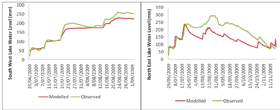
Figure 3. Calibration of lake levels for the South West and North East models.
